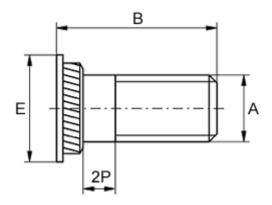
For plate thickness, min = 1.5 Head diameter E = 6 Hole diameter +0.1 = 4.2 Length B = 15 Male thread A = M3x0,5
